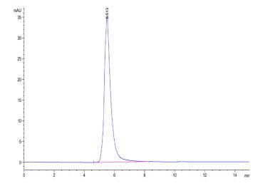
The purity of Human FGFR4 is greater than 95% as determined by SEC-HPLC.
