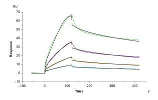
Human FGFR4, hFc Tag captured on CM5 Chip via Protein A can bind Human Beta Klotho, His Tag with an affinity constant of 13.05 nM as determined in SPR assay (Biacore T200).
